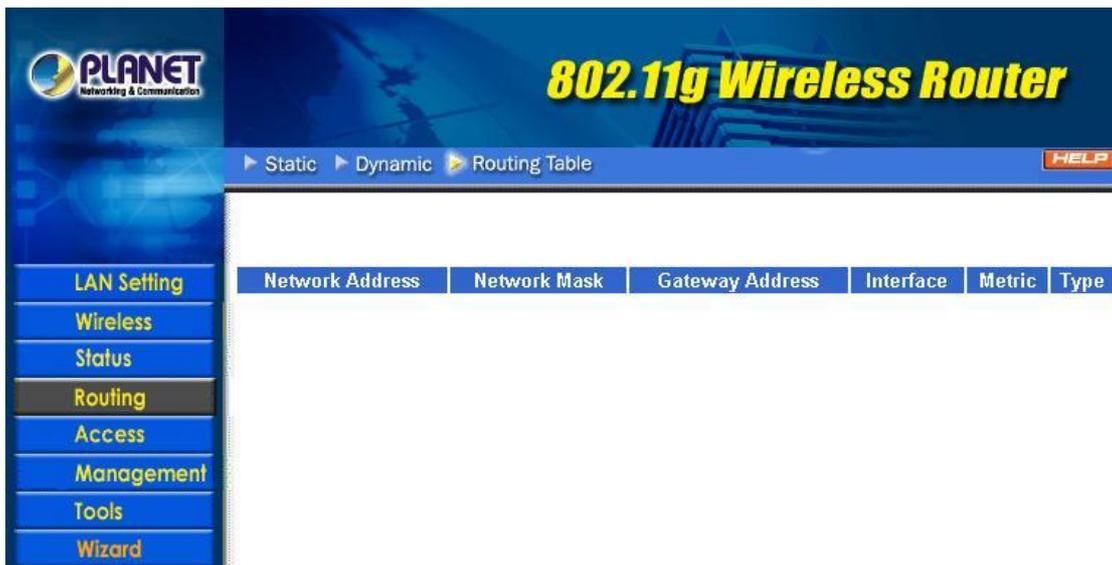
**Network Address:** Displays the network IP address of the connected node.
